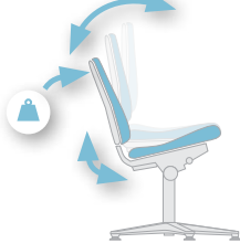
Synchronous mechanism with weight regulation
